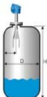
1/3D > R(\text{DN40/50}) > 1/7H ; 1/3D > R(\text{DN80}) > 1/10H ;
